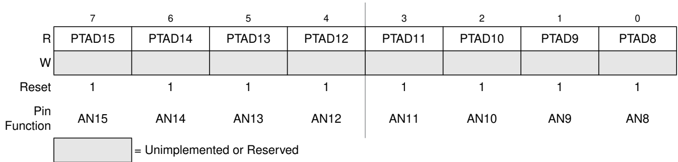
Figure 4-16. Port Data Register 0 (PORTAD0)
