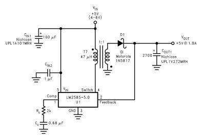
Figure 23. Single-Output Flyback Regulator
