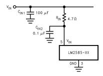
Figure 44. Input Line Filter
