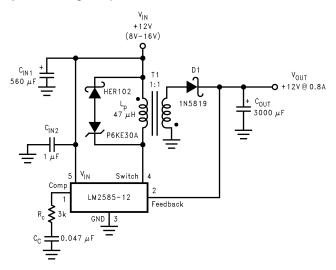
Figure 12. 12-V Flyback Regulator Design Example
