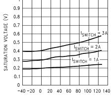
Figure 6. Switch Saturation Voltage vs Temperature
