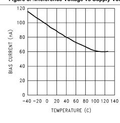
Figure 5. Feedback Pin Bias Current vs Temperature
