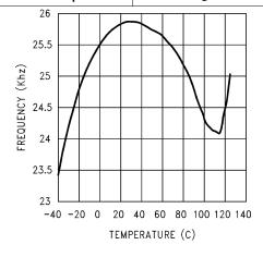
Figure 11. Short Circuit Frequency vs Temperature
