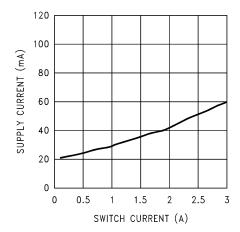
Figure 46. Supply Current vs Switch Current
