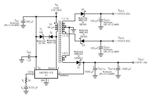
Figure 27. Triple-Output Flyback Regulator
