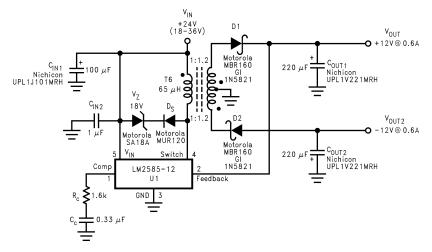
Figure 26. Dual-Output Flyback Regulator
