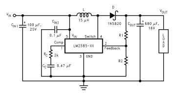
$C_{\text{IN1}}$ —100  $\mu\text{F}$ , 25V Aluminum Electrolytic
