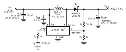
Figure 20. 24-V to 36-V Boost Regulator
