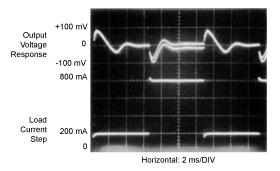
Figure 17. V<sub>OUT</sub> Response To Load Current Step
