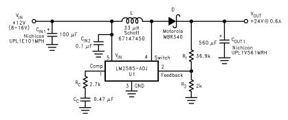
Figure 19. 12-V to 24-V Boost Regulator
