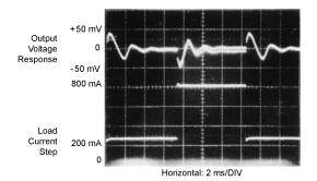
Figure 14. V<sub>OUT</sub> Load Current Step Response
