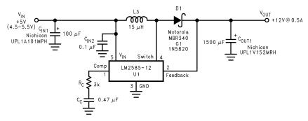
Figure 18. 5-V to 12-V Boost Regulator
