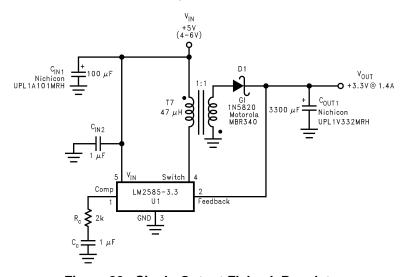
Figure 22. Single-Output Flyback Regulator
