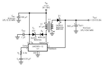
Figure 24. Single-Output Flyback Regulator
