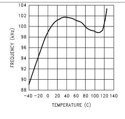
Figure 8. Oscillator Frequency vs Temperature
