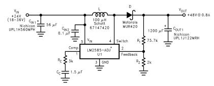
\*The LM2585 will require a heat sink in these applications. The size of the heat sink will depend on the maximum ambient temperature. To calculate the thermal resistance of the IC and the size of the heat sink needed, see *Heat Sink/Thermal Considerations*
