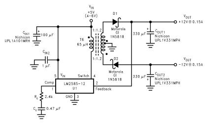
Figure 25. Dual-Output Flyback Regulator
