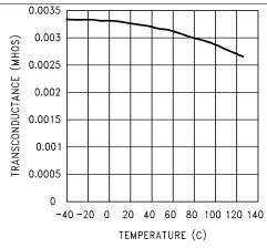
Figure 9. Error Amp Transconductance vs Temperature
