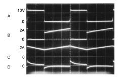
A: Switch Voltage, 10 V/div B: Switch Current, 2 A/div C: Inductor Current, 2 A/div D: Output Ripple Voltage, 100 mV/div, AC-Coupled Horizontal: 2 μs/div
