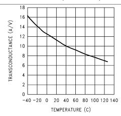
Figure 7. Switch Transconductance vs Temperature
