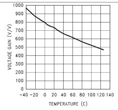
Figure 10. Error Amp Voltage Gain vs Temperature
