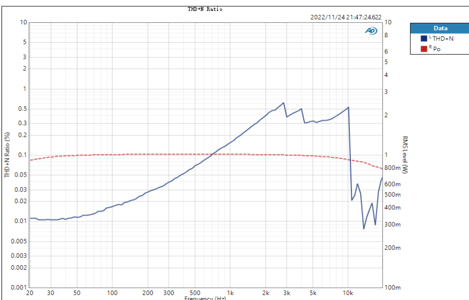
VDD = 12V, P_o = 1\text{W} , frequency vs THD+N
