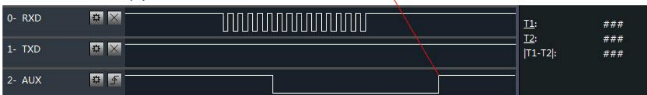
The timing diagram of AUX pin when the module receives serial port data.
