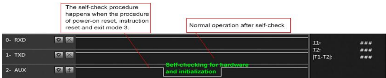
Timing Sequence Diagram of AUX when self-check
