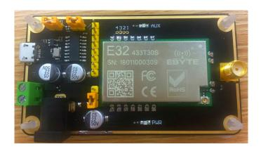
As shown above , connect to jumpers ( 5V power supply , mode 0 ) , both EXX-XXXTBH-01 are configured this way , open serial port , for data TX and RX , and AUX indicator is blinking.
