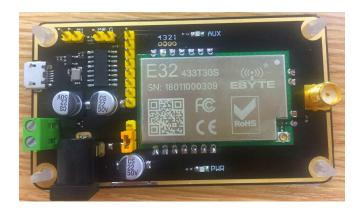
As shown above , connect to jumpers ( 5V power supply , mode 3 ) , see function details from E22 UART module manual.
