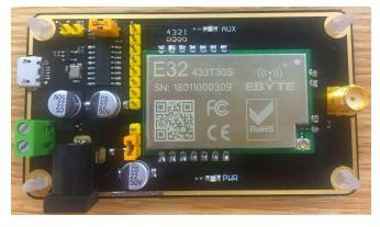
As shown above , connect to jumpers ( 5V power supply , mode 2 ) , see function details from E22 UART module manual.
