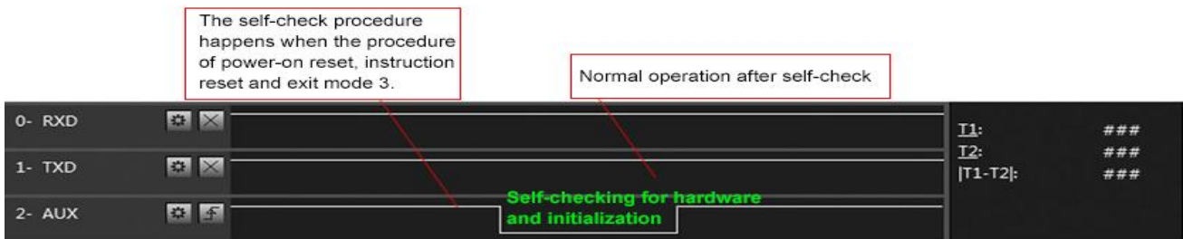
Timing Sequence Diagram of AUX when self-check
