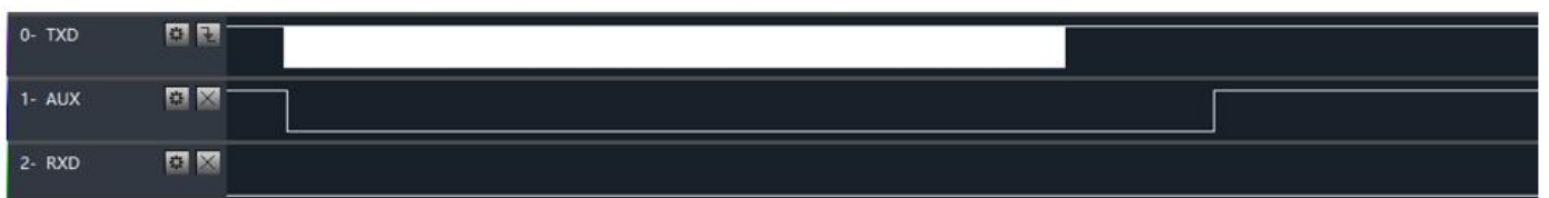
Timing sequence chart of AUX when MCU receives serial data till MCU starts RF transmission
