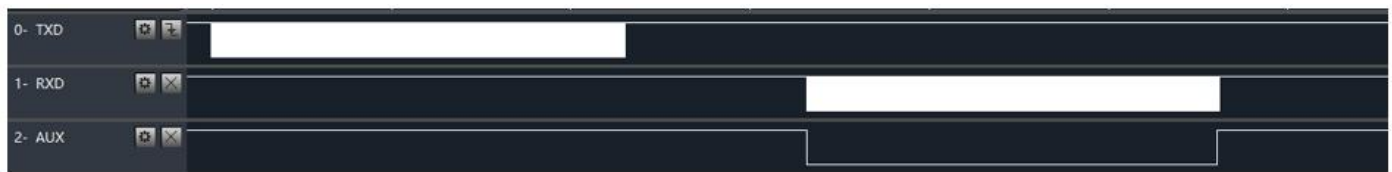
Timing sequence chart of AUX when RF receives data and send to MCU
