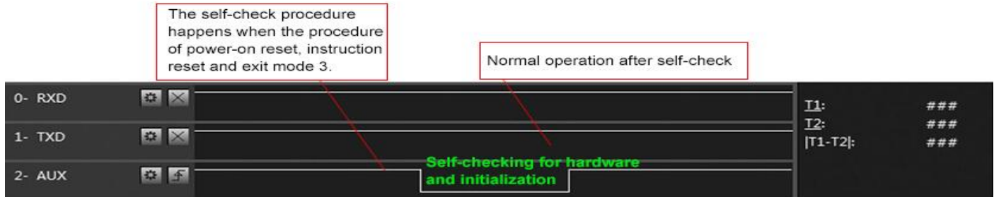
Timing Sequence Diagram of AUX when self-check
