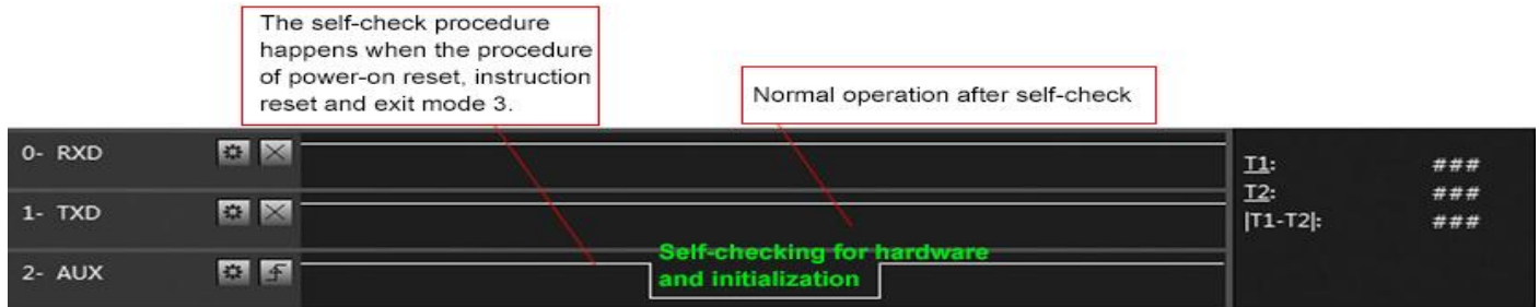
Timing Sequence Diagram of AUX when self-check
