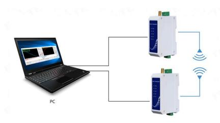
Step4 Install two Serial Port COM test tool on the computer and do a transparent transmission test. Defult parameters for serial port: 9600 baud rate, 8N1 Parity.
