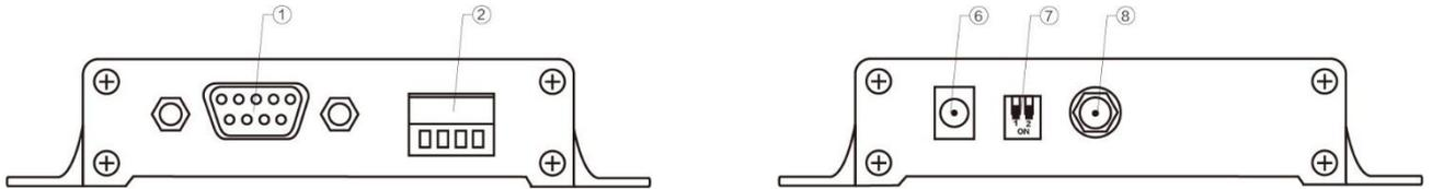
Users can choose ⑥ DC power interface, using the power adapter supply with the interface of the 5.5mm outer diameter , 2.5mm diameter ;
