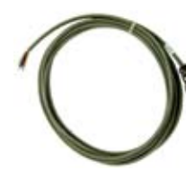
PLC Adapter Cable HMI-CAB-ST001 Connects to AGP3000/ST40x serial port with 9 conductor open ended wires for connecting to 3rd party screw terminal devices.
