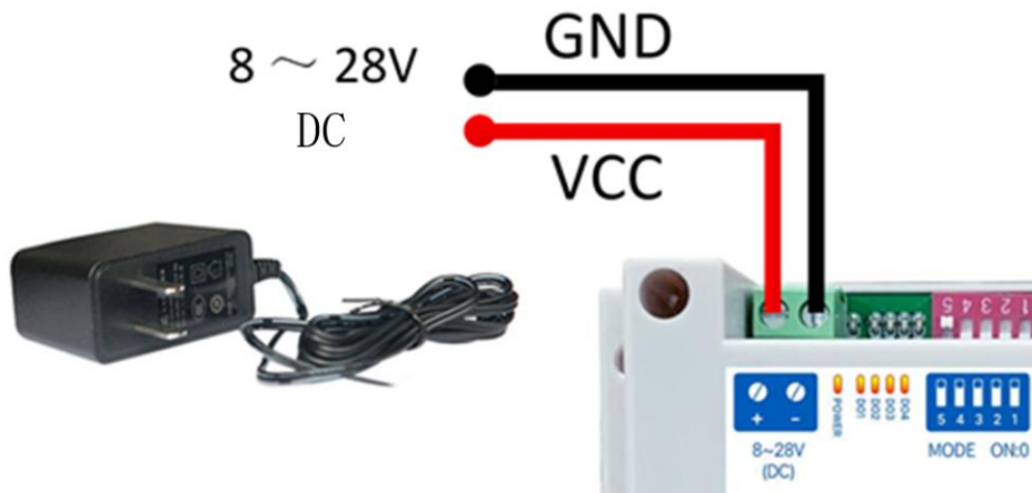
Figure 2-2-1 Power wiring diagram
