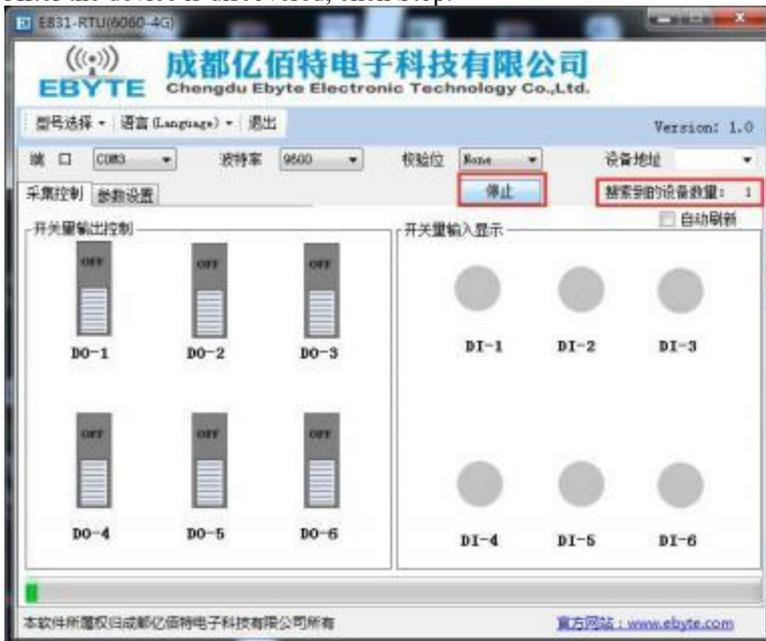
At this time, the device address of the current device can be seen, and the "automatic refresh"  processing can be performed to control the switch output and read the switch input.
