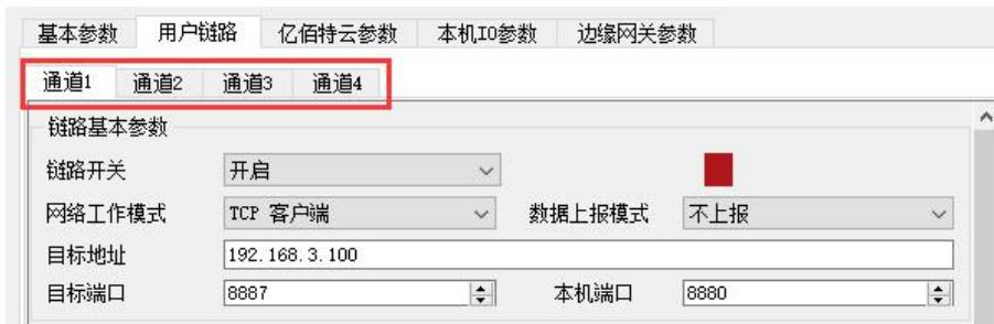
Users do not need to pay attention to the data conversion process between serial port data and network data packets. The device only needs to set simple parameters to realize data transparent communication between the serial port device and the network server.
