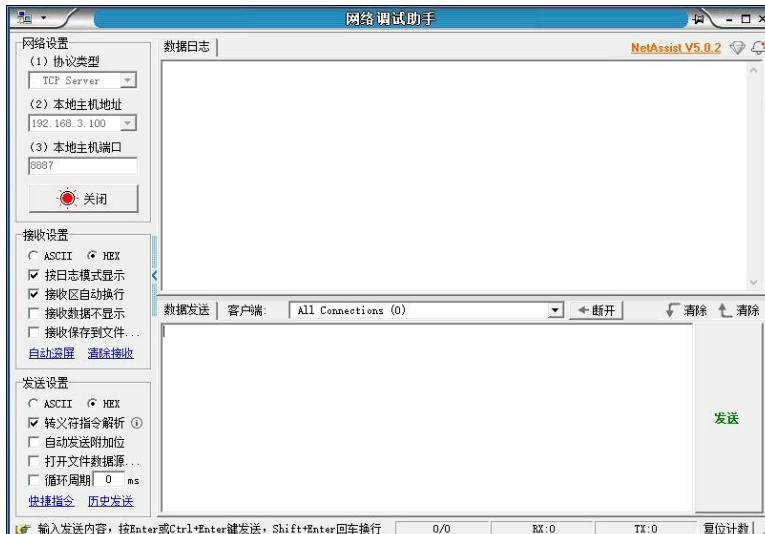
Step 4: Fill in the correct server parameters, configure as TCP client mode, target address, target port, etc., as shown in the figure below:
