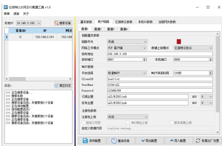
Step 5: After configuring the parameters, save and restart. When the STATE light is always on, the device has been connected to the server platform normally, and wait for the device to report the parameters of the device registration
