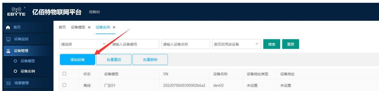
⑤ "Equipment model" select the previously created E870-E0 model, then enter the SN code on the back of the device, fill in other parameters according to your needs, and then click "OK to add" to create the device.
