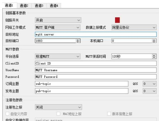
Configure the corresponding subscription publishing address, and use the platform to debug and send data online for communication testing.
