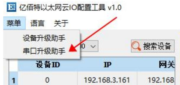
Step 2: Select the serial port number connected to the device, open the serial port, import the upgrade file (the product firmware provided under the corresponding product details on the official website), and click to start the upgrade;
