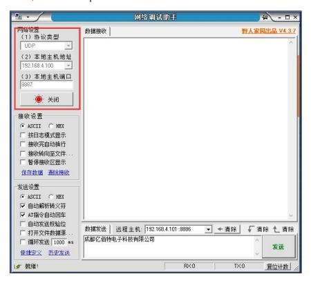
2. Set the network type of SOCKET A1 network type to UDPC (UDP Client), the target IP address is 192.168.4.100, and the destination port is 8887. Click Save to restart the module.
