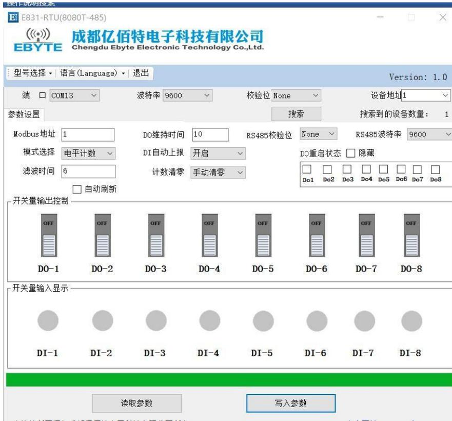
Note, do not check automatic refresh when configuring or reading parameters. Tick auto refresh to read and configure the input and output ports.
