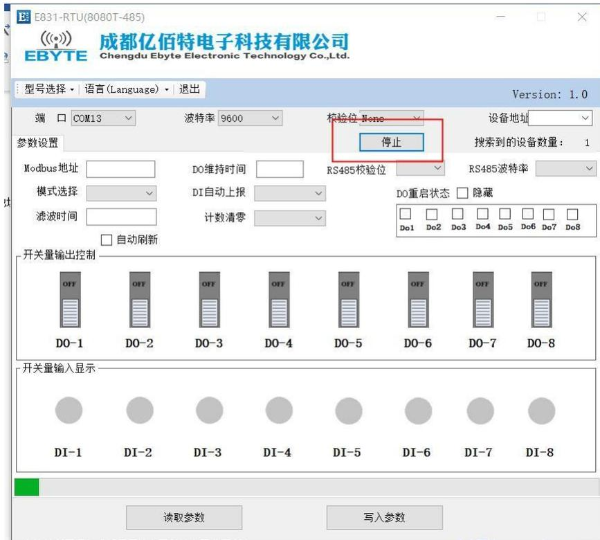
At this time, you can see the device address of the current device, click to read parameters or write parameters, you can read parameters and configuration parameters.
