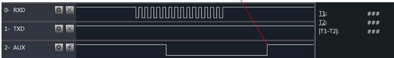
Timing Sequence Diagram of AUX when RXD pin receives
