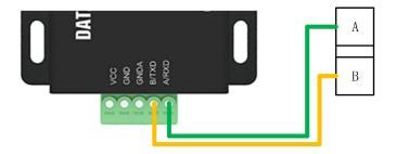
Step 2: Use USB to RS-232,USB to RS-485 or other methods to connect the computer to the digital radio;
