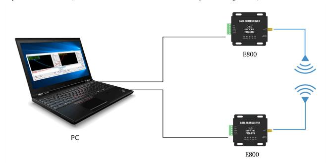
Step 3: Start two serial port debugging assistants, select the serial port baud rate as 9600bps and the verification method as 8N1, then the serial port transparent transmission can be realized;
