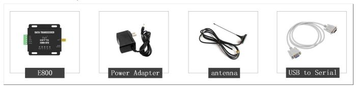
Step 1: First install the antenna for the data transmission, then turn on the power, and connect the USB to serial cable (USB to RS485);
