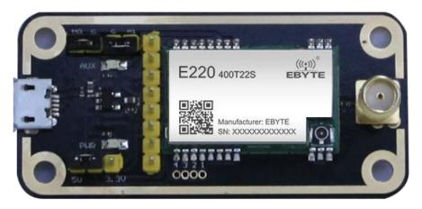
As shown above, connect to jumpers (5V power supply, mode 0), both EXX-XXXTBL-01 are configured this way, open serial port, for data TX and RX, and AUX indicator is blinking.
