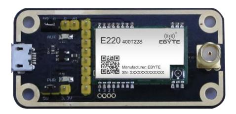
As shown above, connect to jumpers (5V power supply, mode 2), see function details from E22 UART module manual.
