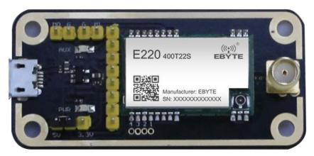
As shown above, connect to jumpers (5V power supply, mode 3), see function details from E22 UART module manual.
