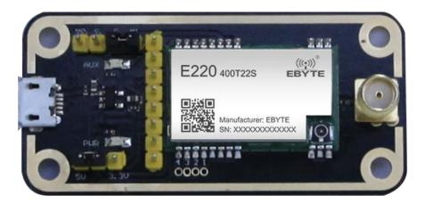
As shown above, connect to jumpers (5V power supply, mode 1), see function details from E22 UART module manual.
