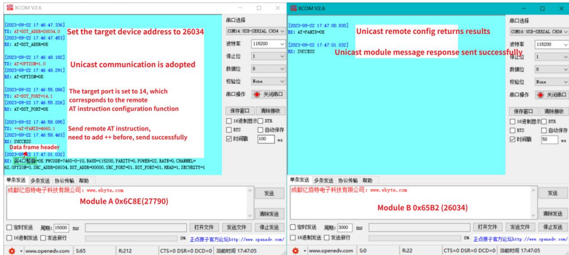
Figure 8.2.1 Remote single point configuration steps
