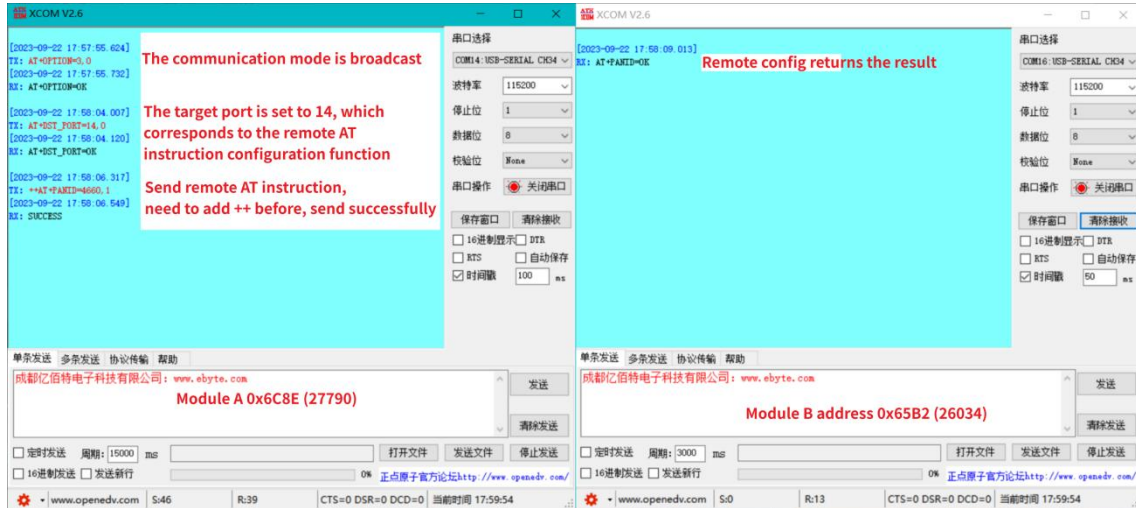
Figure 8.3.1 Remote broadcast configuration steps
