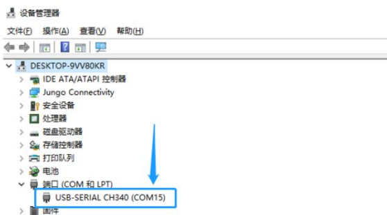
Figure 5.1.2 Device Manager checks COM port
