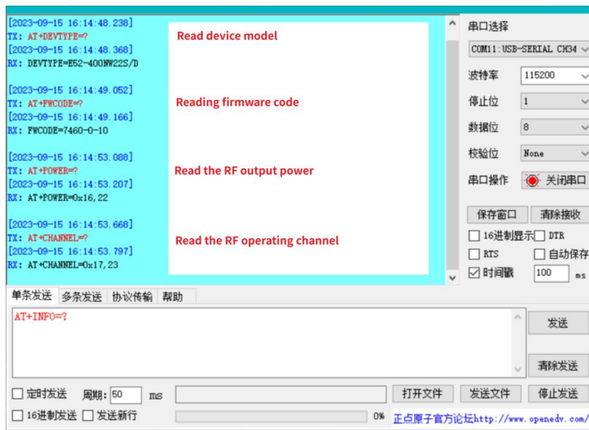
Figure 8.1.2 MCU obtains parameters
