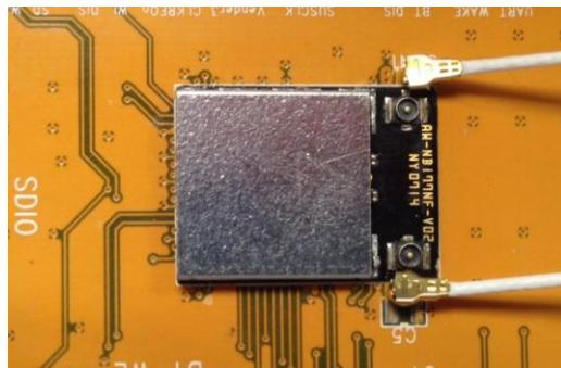
Step 3. Unmount the NGFF1216 module from motherboard by soldering.
