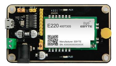
As shown above, connect to jumpers (5V power supply, mode 1), see function details from E22 UART module manual.
