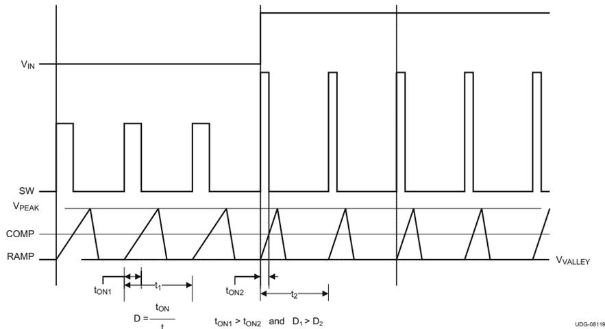
**Figure 7-1. Voltage Feedforward Effect on PWM Duty Cycle**
