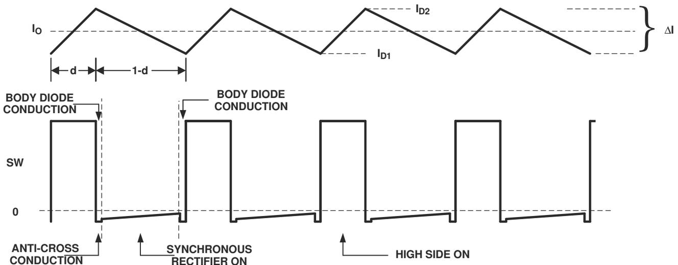
**Figure 8-1. Inductor Current and SW Node Waveforms**
