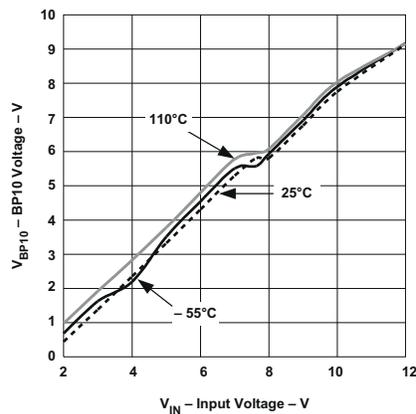
**Figure 6-5. Input Voltage vs BP10 Voltage**
