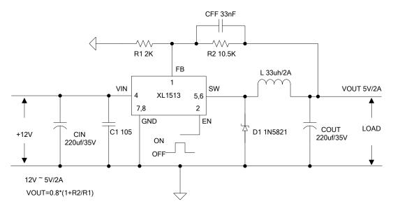
Figure 7. XL1513 System Parameters Test Circuit (12V ~ 5V/2A)
