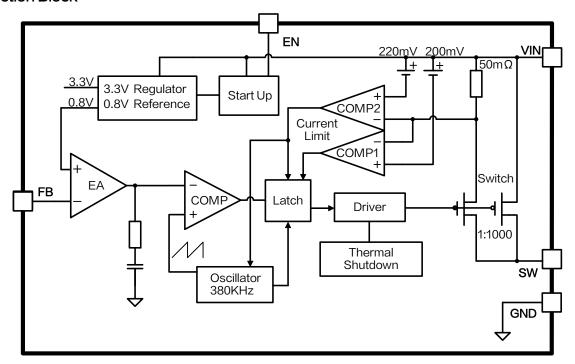
Figure 3. Function Block Diagram of XL1513
