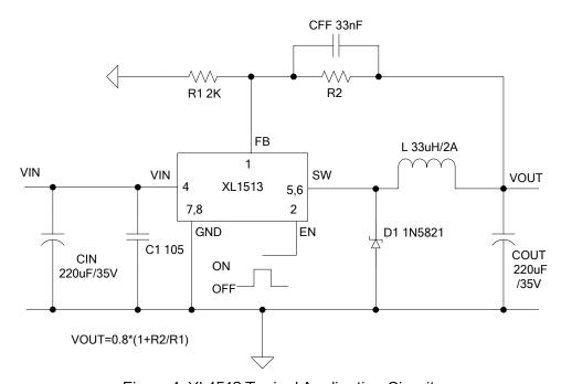
Figure 4. XL1513 Typical Application Circuit
