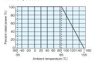
For resistors operated at an ambient temperature of  $85^{\circ}\mathrm{C}$  or higher, the power shall be derated in accordance with the above derating curve
