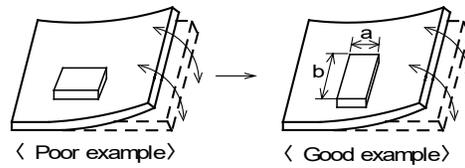
(2) Components location on PCB separation
