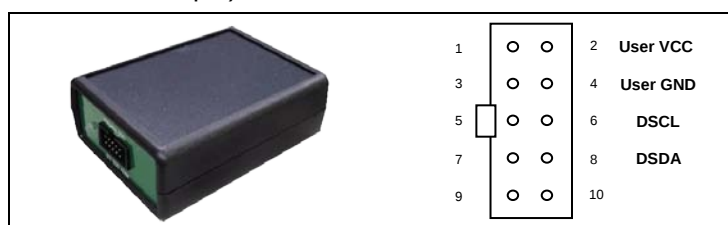
Figure 1-1 On Chip Debugger 2 and Pin description (ocd2 mode)
