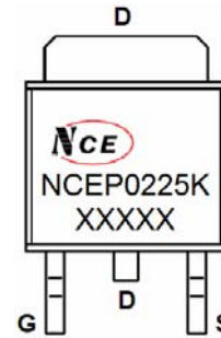
Marking and pin assignment
